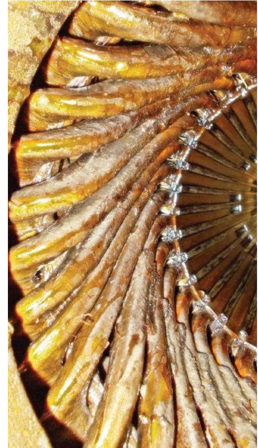
Melted motor windings at Hualalai Source: SME TDI Report, Sept. 2016
